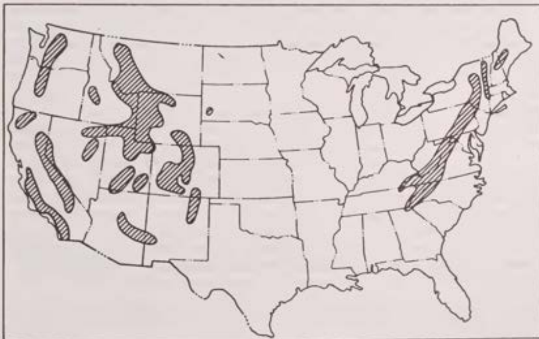
FIGURE 2.—Regions where precipitation management may be applied to enhance snowfall from winter orographic weather systems, thus augmenting spring and summer runoff from mountain snowpacks.
