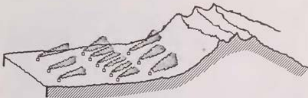
FIGURE 6.—Schematic view of silver iodide generators placed upwind from a target area in the mountains, where orographic clouds are to be seeded for precipitation enhancement. (From Weisbecker, 1974.)
