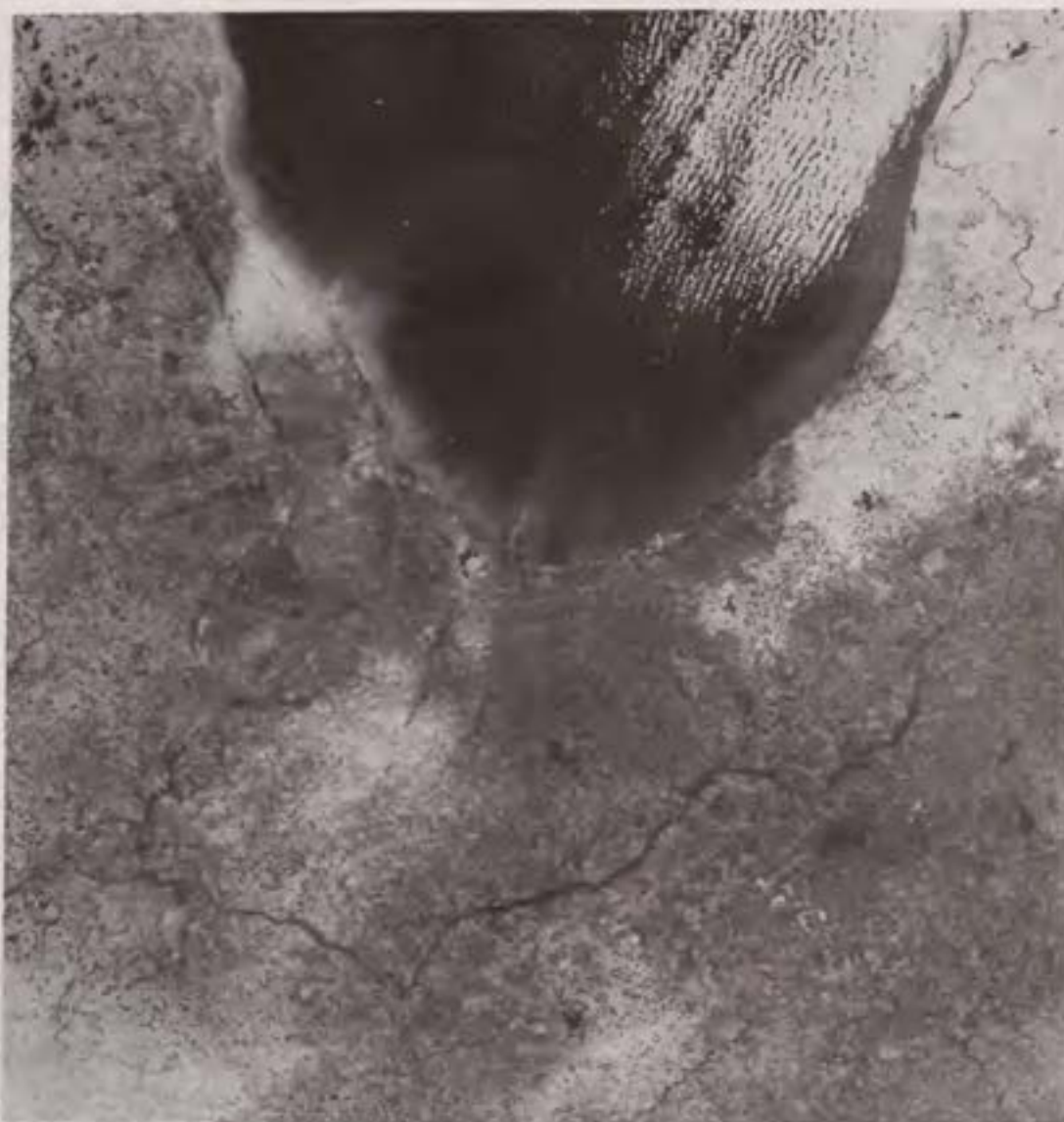
FIGURE 6.—The formation and building of clouds can be influenced by the presence of pollutants acting as nuclei upon which water vapor condenses and by the hot dry air with which these aerosols are swept aloft. In this Landsat photo, excess particles as well as heat and moisture produced by the industries of Gary, Ind., favor the development of clouds downwind. The body of water shown is the southern tip of Lake Michigan. (Courtesy of National Aeronautics and Space Administration.)
