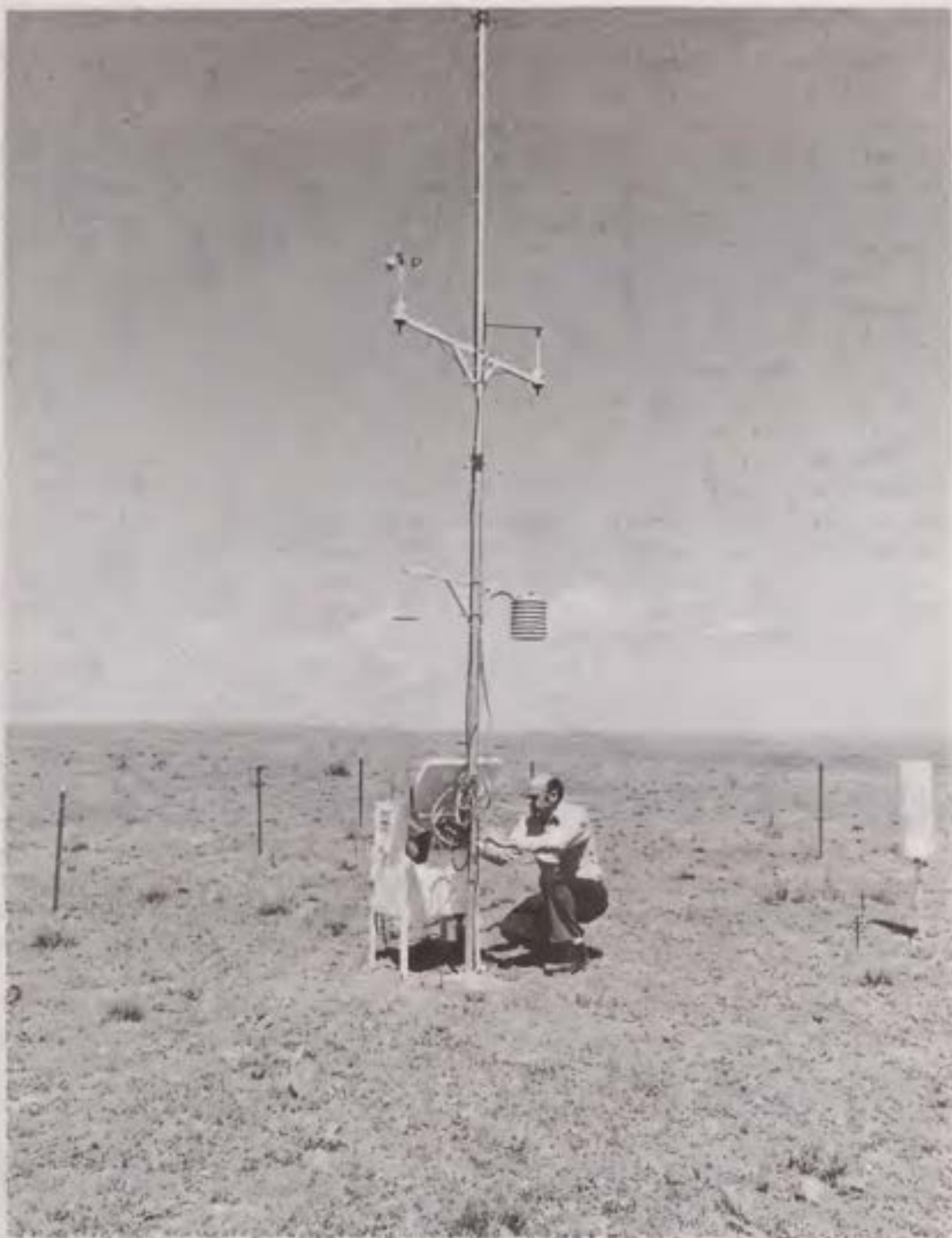
A typical remote field installation of the portable automated mesonet (PAM) system. (Courtesy of the National Science Foundation.)
