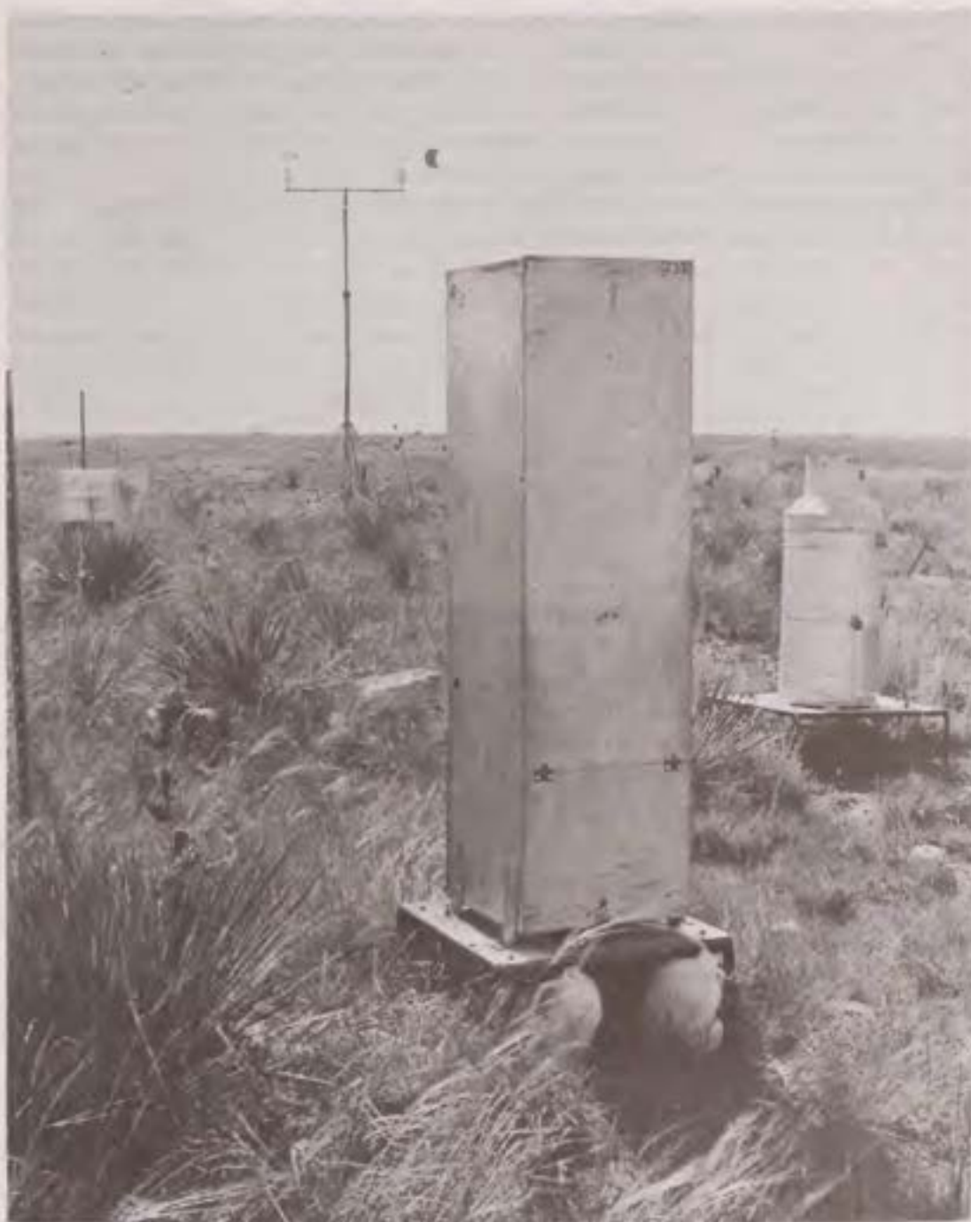
Precipitation instrument site, including, from left to right, hailcube, anemometer, rain/hail separator, and Belfort weighing precipitation gage. (Courtesy of the National Science Foundation.)
