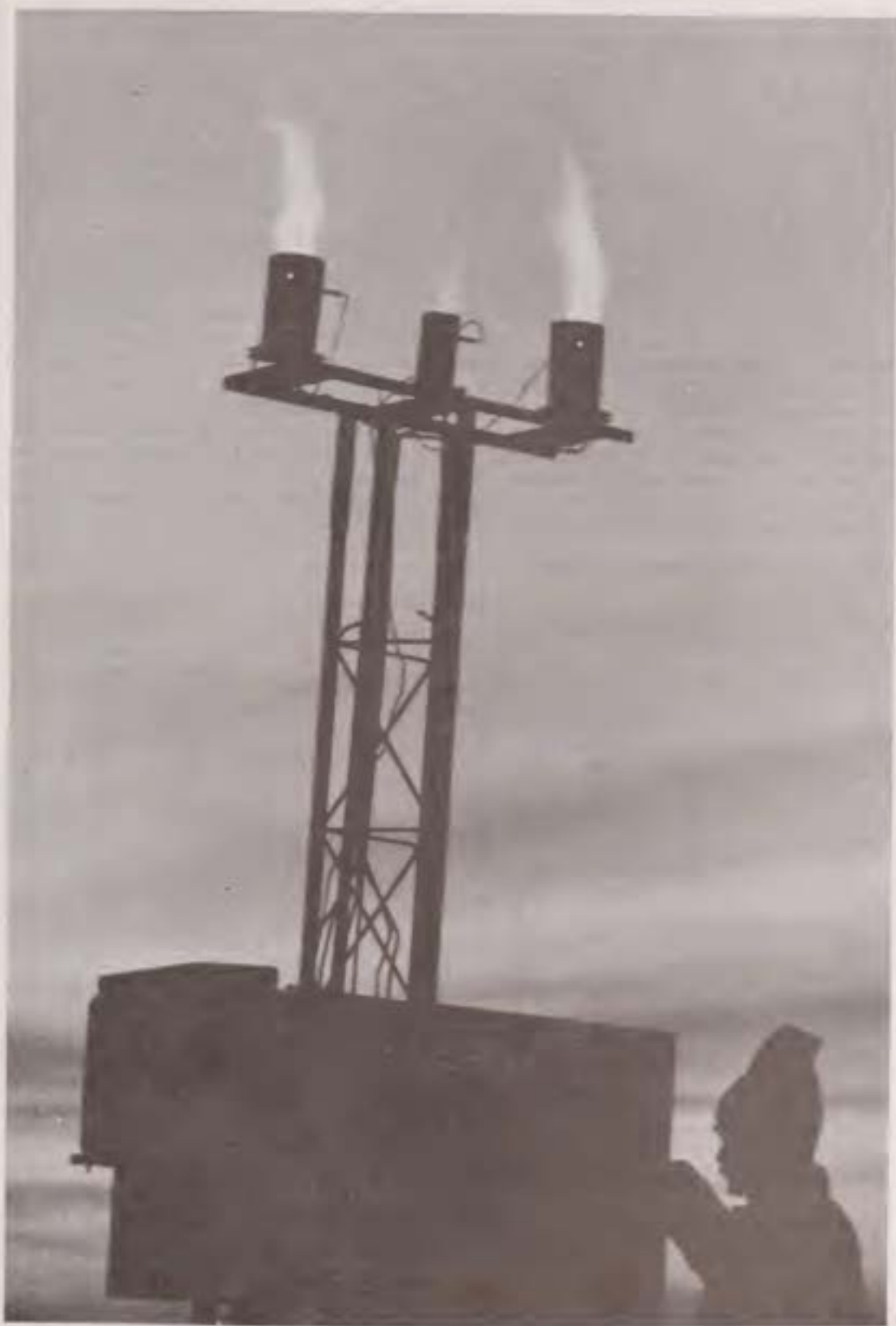
Manually operated cloud seeding generator similar to those used in the Colorado River Basin Pilot Project. (Courtesy of the Bureau of Reclamation.)
